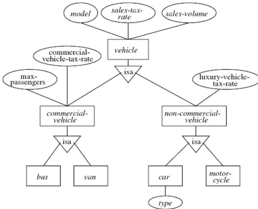
Figure 2.19 E-R diagram of motor-vehicle sales company.
